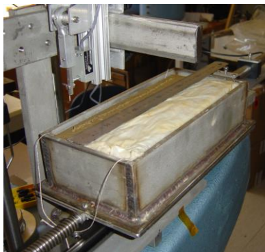
Fig. 2. An example of an experimental cut of saturated plastic soil.
